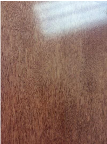
Figure 4 - Acrylic High-Solids UV-Cure Clear Wood Finish Filled with 5 μm N.S. at 10 % by Wt. Based on Resin Solids over Stained Maple Veneer (DFT = 3mil).
